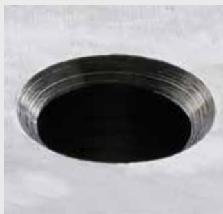
Countersinking with standard countersink
